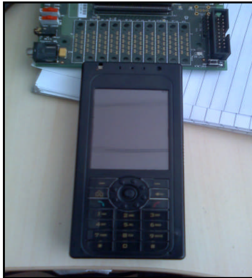
Figure 3 PXA310 Handheld Platform Development Kit [Littleton]
