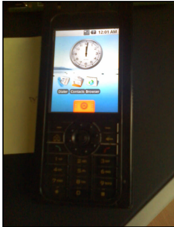
Figure 8 Android Running On the PXA 310 Handheld Platform Development Kit
